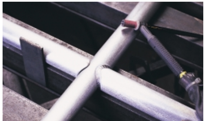
Narrow beads like this — created with the Dynasty inverter — take 25% less time to weld and 15% less time to polish.
