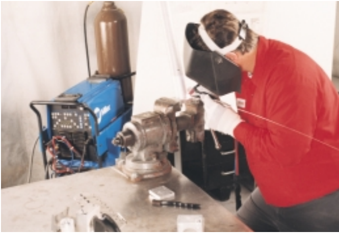
The Dynasty™ inverter eliminated arc instability and arc wandering, improving weld quality on these small, aluminum airplane components.
