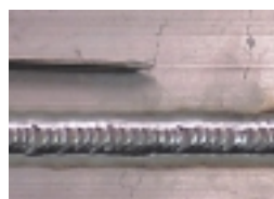
Extending the Dynasty's balance control to 90% EN narrowed the etched zone.
