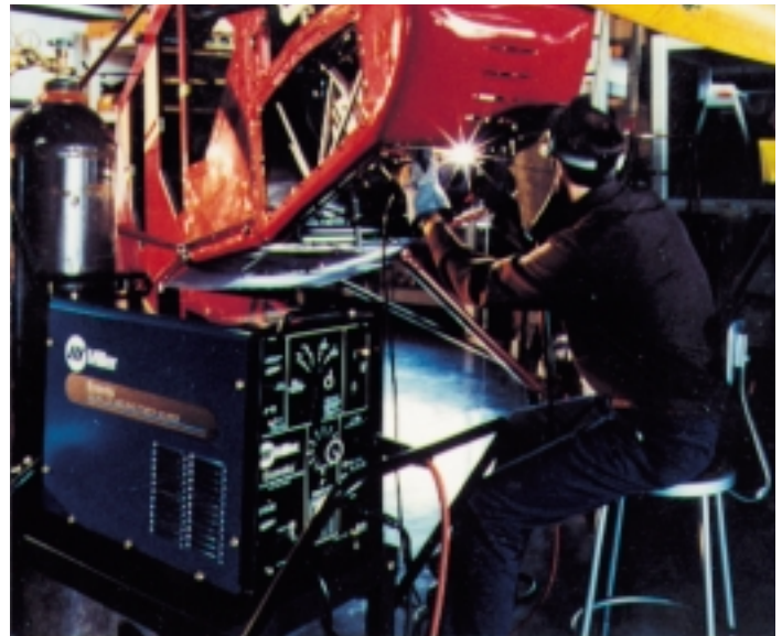
Designed for hobby work, Miller's Econotig® creates AC and DC arcs for TIG and Stick welding.
